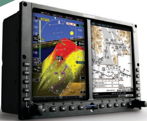
Garmin's SVT™ 3-D synthetic vision renders terrain-alerting data into a realistic virtual landscape, showing obstacles, traffic, airports and more. A scaled version of SVT is standard on the
